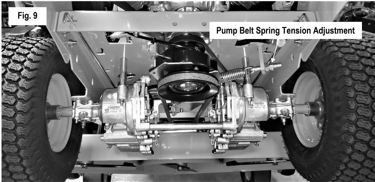
The tension should be adjusted so that there is between 60 to 65 lbs. of tension on the belt and recheck belt tension after half an hour. This can be checked with a belt tension gauge (Part Number 041-9999-00) as shown in Fig. 10.
