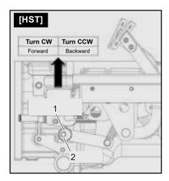
(1) Neutral Adjust Shaft (B) Fix Bolt
