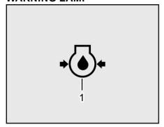
(1) Engine Oil Pressure Warning Lamp
